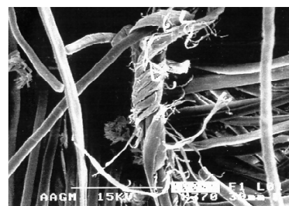
Figure 10. A broken fibre end on dry-cleaned fabrics.
