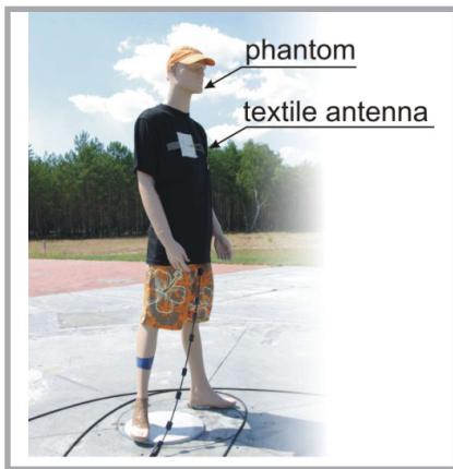
Figure 7. Antenna placed on phantom for radiation pattern measurements at open-field antenna test facility.
