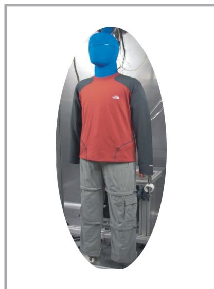
Figure 2. Fabric sweating thermal manikin “Walter”.
