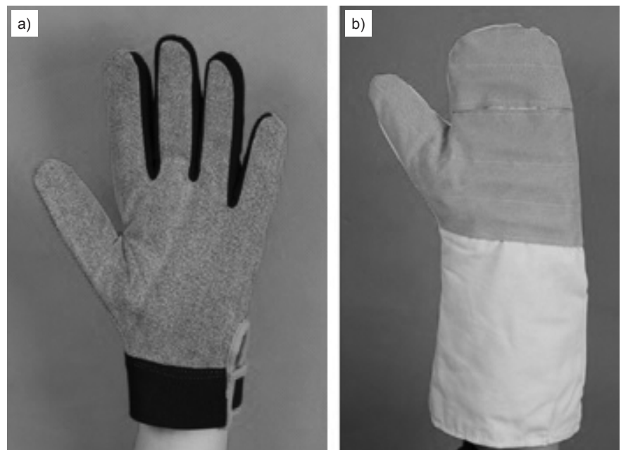
Figure 1. Examples of glove designs determined by type of hazard: a) fitted gloves made of polyamide fibres highly resistant to cuts, protecting against light and moderate mechanical injuries, b) large mittens made of several layers of fabrics including an insulating heat-resistant nonwoven (source CIOP-PIB).
