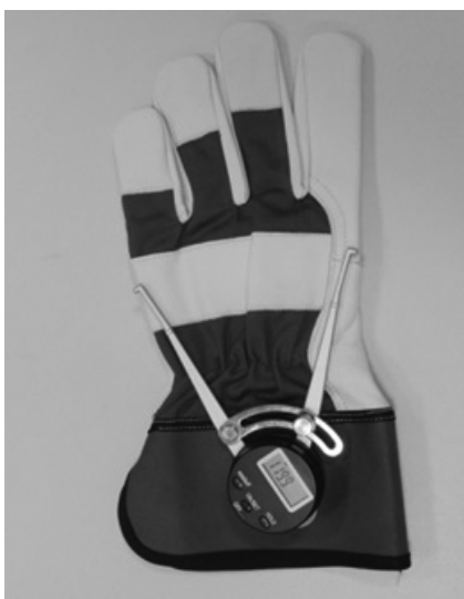
Figure 4. Digital inside caliper used for measuring the internal dimensions of protective gloves.
