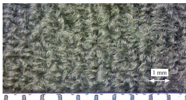
Figure 3. BCP/PU complex knitted fabrics made of BCP/PU complex yarns. The BCP/PU complex yarns were fabricated with 77 dtex polyurethane fibres and 70D bamboo charcoal polyamide textured yarn. The wrapped counts of the BCP/PU complex yarns were 200 turns/m, the expanded multiple of the polyurethane fibres - 3, and the speed of the rotor twister was 4000 r.p.m.
