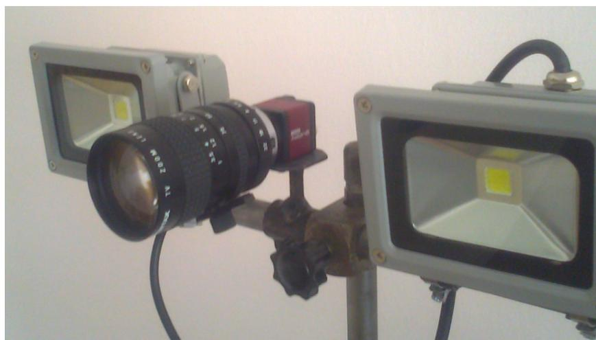
Figure 1. Photo shoot setup (System via CCD camera).
