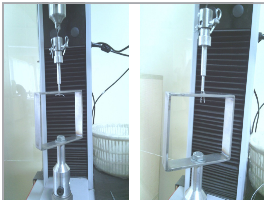
Figure 5. Photo of the stiffness tester (Testometric M250-2.5 CT Modified).
