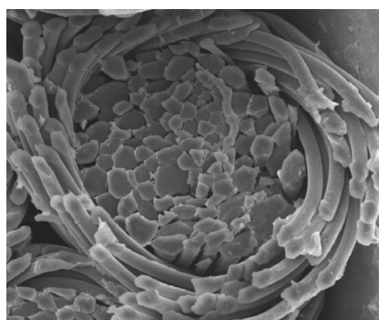
Figure 11. Cross section of yarn: FLAX/PLA (Core-Flax) 100 tex, Hollow spindle spinning technique.
