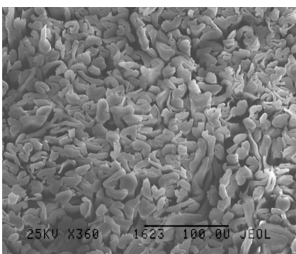
Figure 9. Microscopic pictures of fibre cross-sections: a) Turkish light brown long (TLBL), b) Turkish green (TG).
