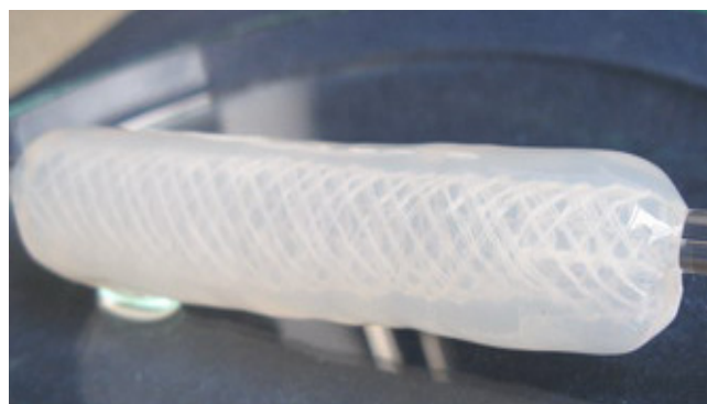
Figure 4. Prototype of a prosthesis obtained in a reactor with a rotating shaft and the polyester vein reinforcement applied - BR-1 (Tricomed SA).
