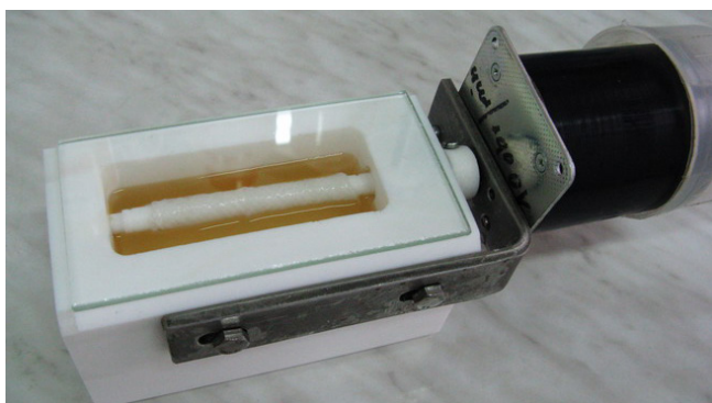
Figure 3. Dynamic culture in a reactor with a rotating PTFE shaft and the polyester vein reinforcement applied - BR-1 (Tricomed SA).
