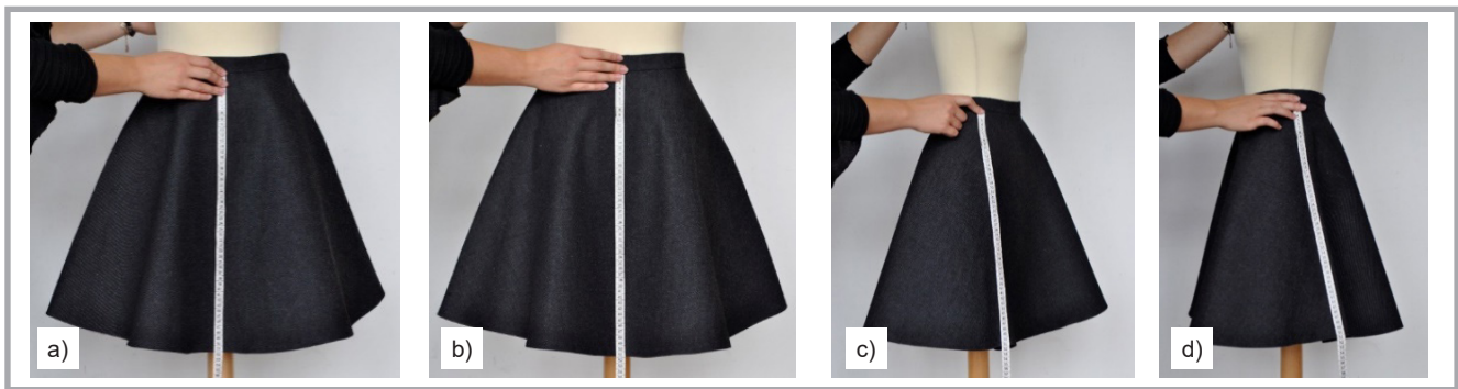
Figure 1. Presentation of measuring draped real flared skirts' lengths; a) front, b) back, c) right, d) left.
