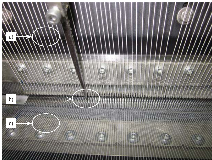
Figure 2. Schematic of elastic warp-knitted fabric; a) rubber thread, b) front feeder, c) PET warp yarn.
