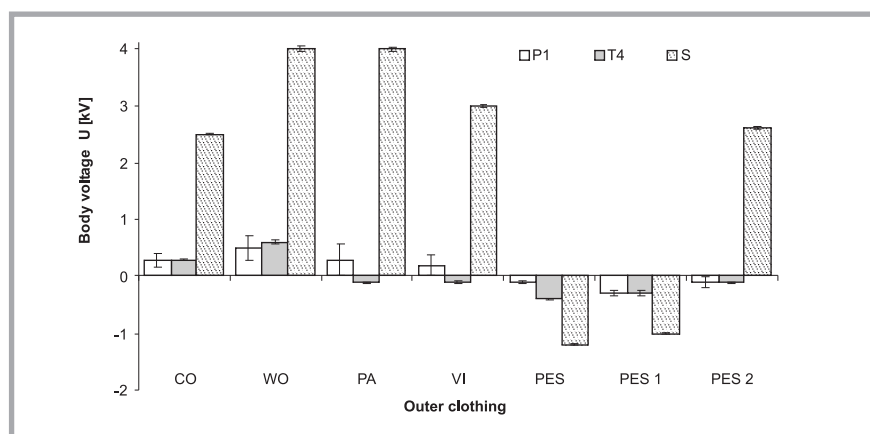
Figure 4. Means of maximum values of the operator's body voltage while using a chair covered with different textile upholstery materials.
