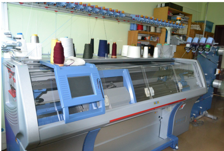
Figure 1. Computer controlled flat knitting machine CMS Stoll.
