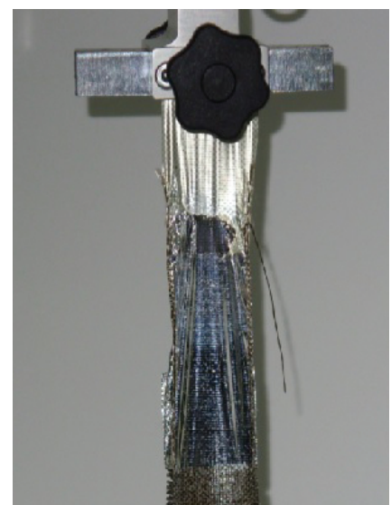
Figure 5. Strong adhesion between the aluminum foil and basalt fabric – L4.
