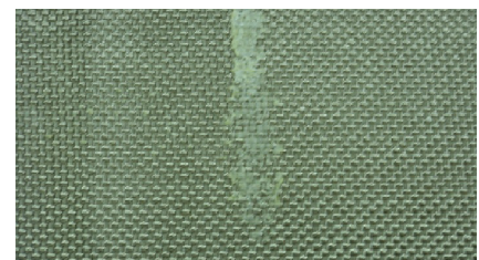
Figure 3. Glue layer visible on the right side of fabric – L4
