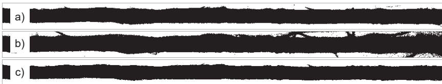
Figure 10. Comparison of yarn segmentation results and computation time; a) result by Otsu's thresholding: 0.21 s, b) result by FCM clustering: 1.14 s, c) result by region growing algorithm: 6.33 s.
