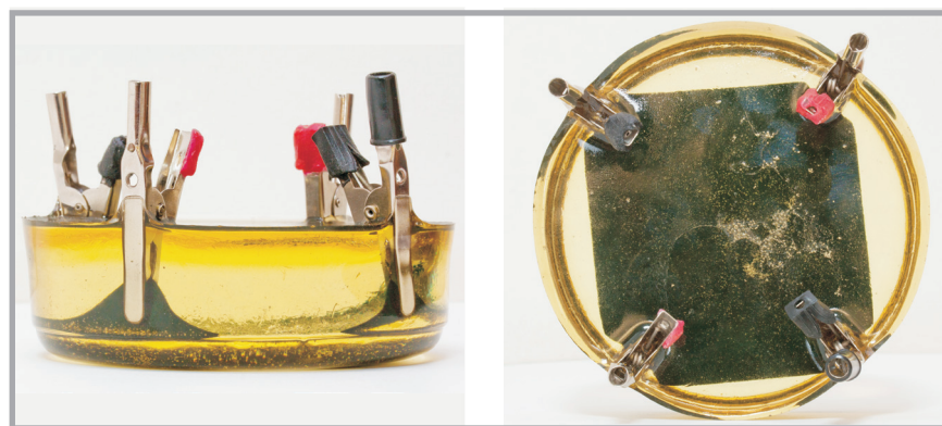
Figure 1. PPy coated fabric sample potted in transparent epoxy, with integrated contacts for VDP measurements. Side view (left) and top view (right).
