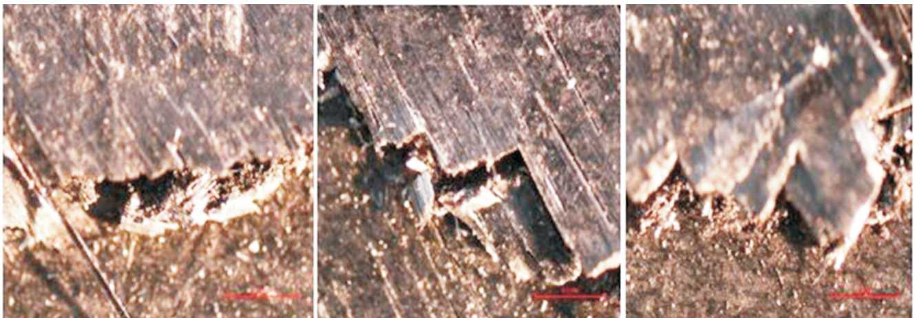
Figure 9. Optical microscope photos for Un1, Un2, and Un3: [45/45/90/0]_{2s} .
