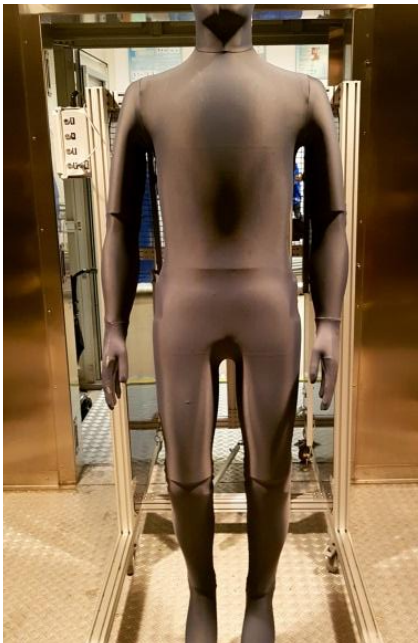
Figure 4. Thermal manikin dressed in special skin.
