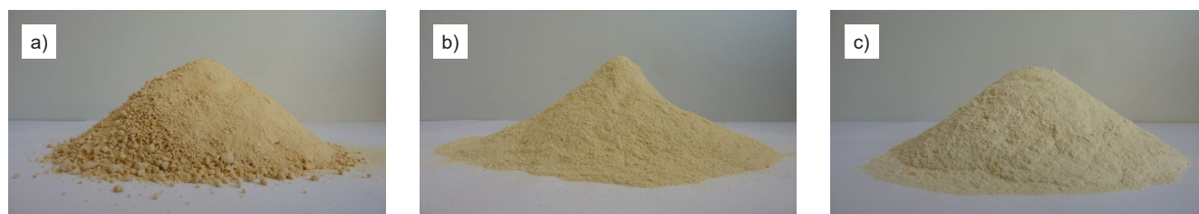
Figure 1. Intermediates obtained from modification of starch-protein raw materials: a) chemically esterified intermediate, Q-Farin C1000, DS = 0.7, b) oxidized intermediate Q-Farin C1000, DO = 1.2%, c) enzymatically esterified intermediate Q-Farin C1000, DS = 0.2.
