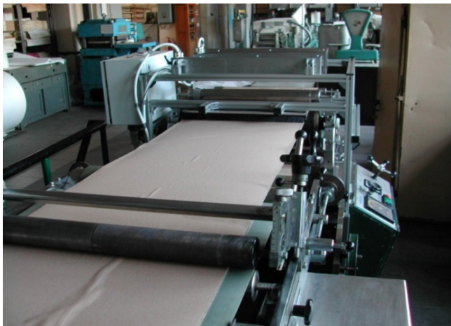
Figure 6. Experimental setup for the production of corrugated cardboard.
