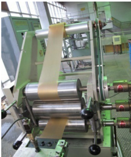
Figure 2. Plasti-Corder® 330 apparatus with a single screw extruder.
