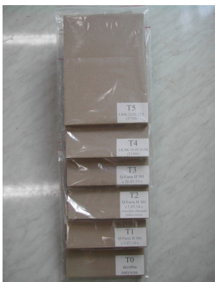
Figure 7. Samples of corrugated cardboard made with the use of the adhesives developed.
