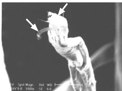
Figure 7. Tip fibrillation (grey fibre).
