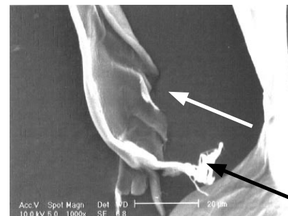
Figure 2. End rupture (grey fibre).
