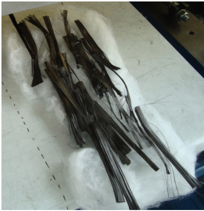
Figure 2. Fibre materials (80 mm virgin staple CF and PA 6) before feeding into the carding machine in the case of manually oriented virgin staple CF.
