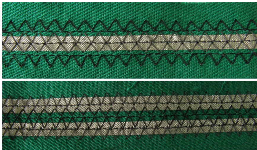
Figure 4. Example of the new kind of textile transmission line (top and bottom view).
