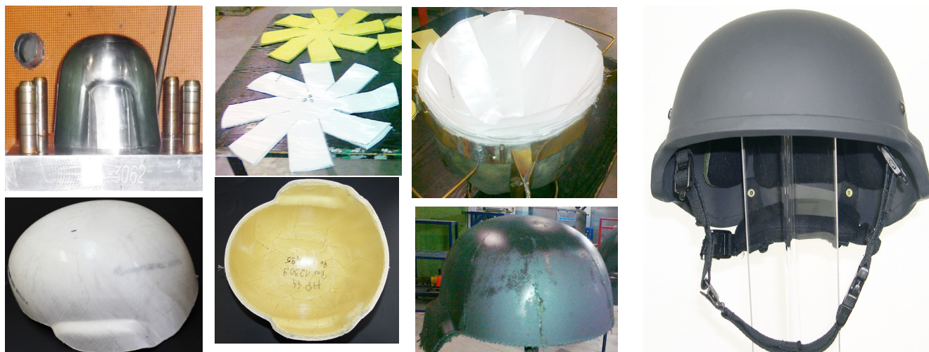
Figure 6. Photographic documentation depicting the steps of ballistic hybrid helmet fabrication.
