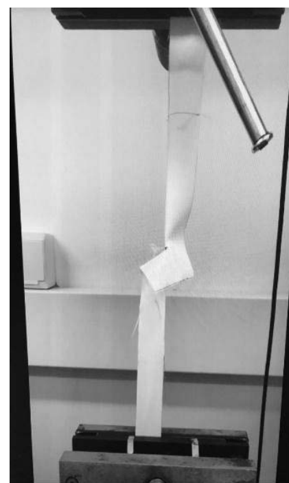
Figure 3. View of tearing test.
