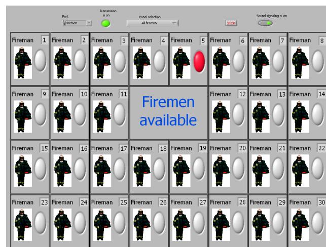
Figure 6. Panel of the centre program - all the firemen are monitored simultaneously; the pane included signal lamps for 30 firemen
