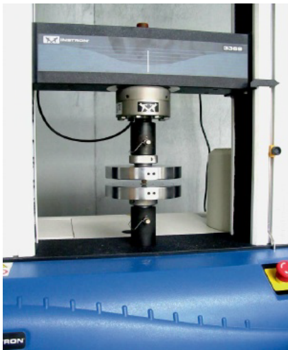
Figure 2. Schematic of Instron Universal Testing Machine (Model 3369).
