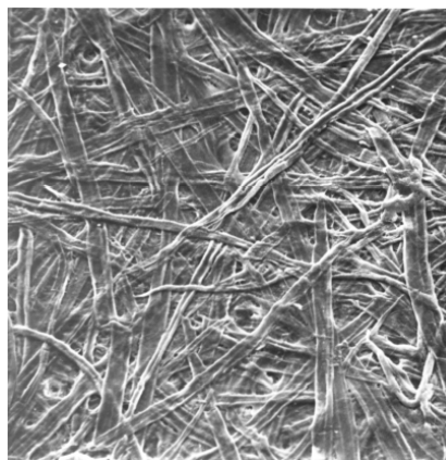
Figure 1. Microscope image of a paper surface of approx. 1 mm 2 [14].
