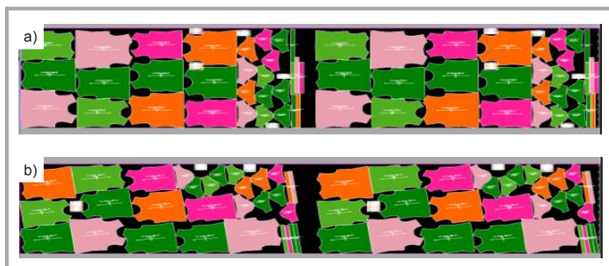
Figure 6. a) Marker layout plan (12 sizes) – no spirality and b) marker layout plan (12 sizes) – 7% spirality rate.
