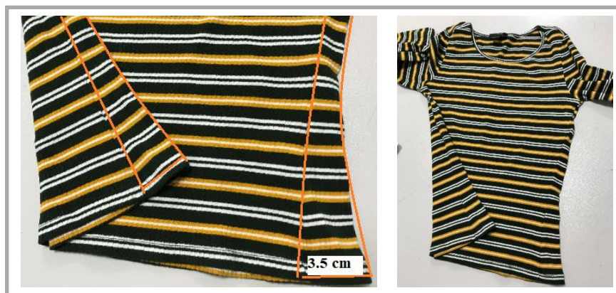
Figure 5. Example of a garment with faulty fabric spirality.
