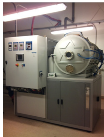
Figure 1. Magnetron device (general view).
