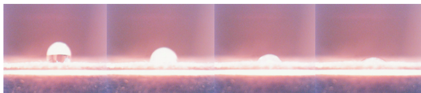
Figure 1. Change in time of the drop profile on the surface of the PET textile in 150 seconds.
