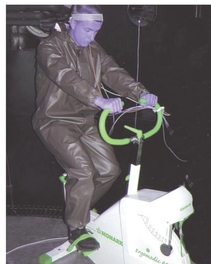
Figure 2. Testing of protective clothing in a climatic chamber.
