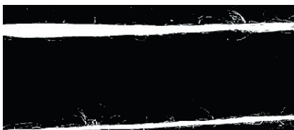
Figure 6. Flax yarns wet spun with false twist.
