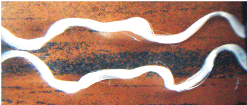
Figure 6. Aspect of PES HT yarns after deknitting.
