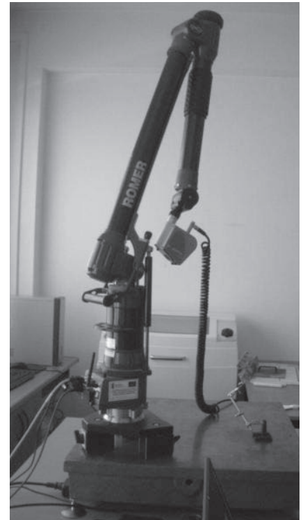
Figure 4. Romer CimCore Ininity 2 measuring arm with scanning head contour probe.
