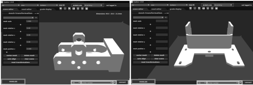
Figure 12. Elements of warp guide bars of fabric sidewall – programming the 3D printing process (Voxelizer software).
