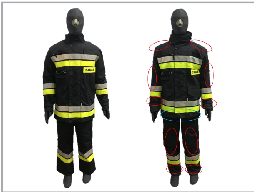
Figure 2. Sample of firefighter personal protective clothing (FFPPC) (from left: EN_1, EN_2) with the place with the difference in the construction of the clothes marked.
