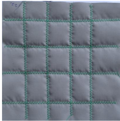
Figure 5. Prepared multilayer package quilted using a zig-zak stitch and 80 tkt thread after the sixth step of quilting.
