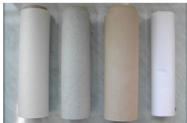
Figure 11. Photo of PP/DM composite nonwovens (from the left: PP/F, PP/WP, PP/MDF, PP/CF).
