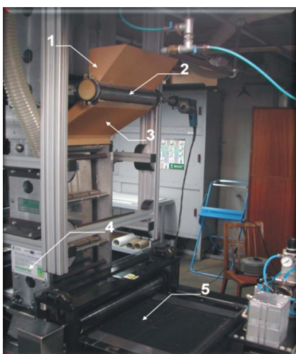
Figure 2. Fragment of a spun-bond installation with a dosing system: 1 – charging hopper, 2 – feed roller, 3 – inlet channel, 4 – disturbance channel, 5 – transport sieve.
