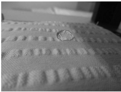
Figure 3. Drop of water on the surface of grey seersucker woven fabric after the test of moisture management using the MMT.
