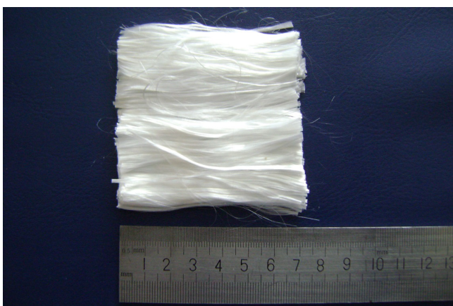
Figure 2. Picture of TEXZEM PES 200 polyester fibres from Bonar Geosynthetics a. s. [8].
