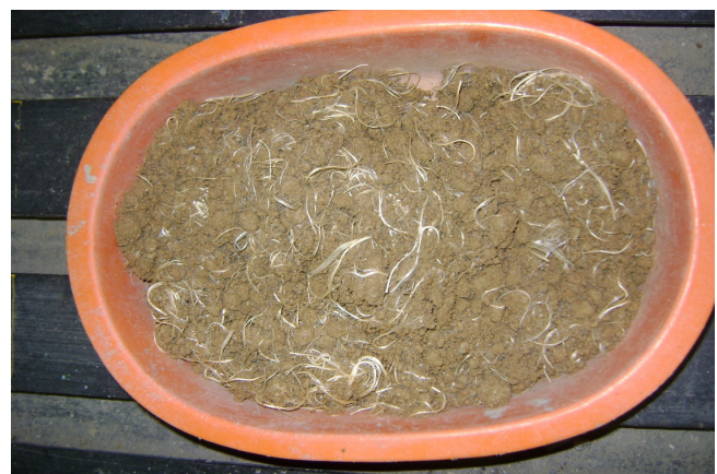
Figure 3. Part of specimen of soil CS mixed with 0.5% of fibres before compaction into a shear box.
