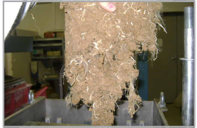
Figure 5. Effect of fibres in a cohesion increase (soil CS, 1.0 % of fibre).
