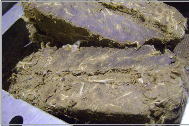
Figure 4. View of the shear zone after the test of soil CH with 1% of fibres.
