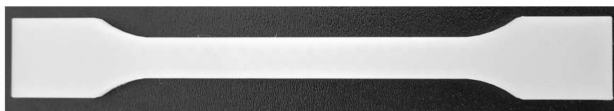
Figure 1. Specimen printed for tensile tests.
