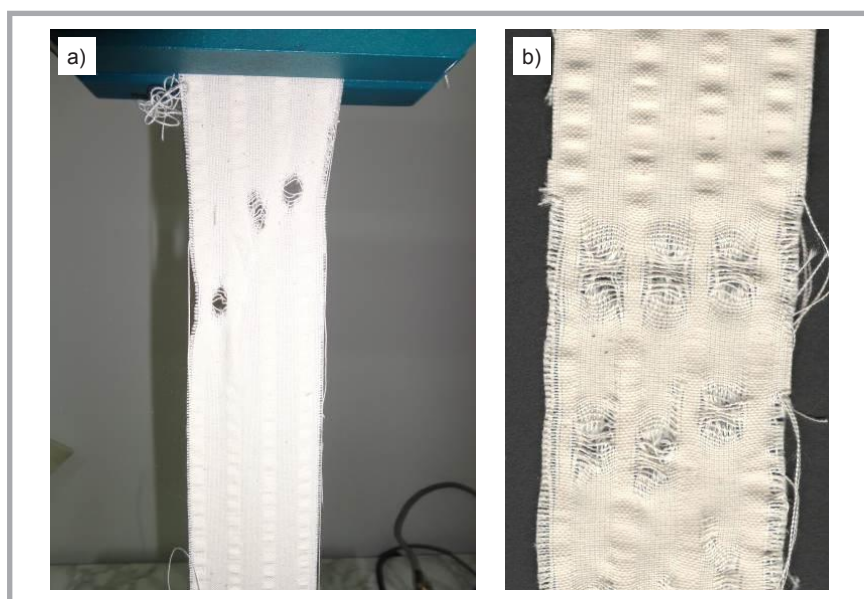
Figure 6. Breaking of seersucker fabrics in the warp direction: a) sample mounted in the clamps of the tensile tester; b) scan of broken sample.
