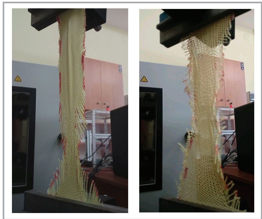
Figure 4. Pictorial presentation of bias tensile tests: a) biaxial and b) triaxial samples under tension on an Instron.
