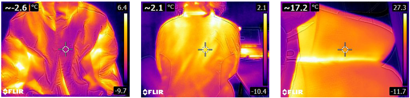
Figure 2. Thermograms of individual 2, Phase One: a) chest, b) back, c) thighs.
