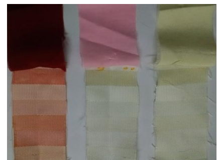
Figure 10. Colour staining in multifibre test sample tested with dyed silk fabrics in perspiration fastness testing.
