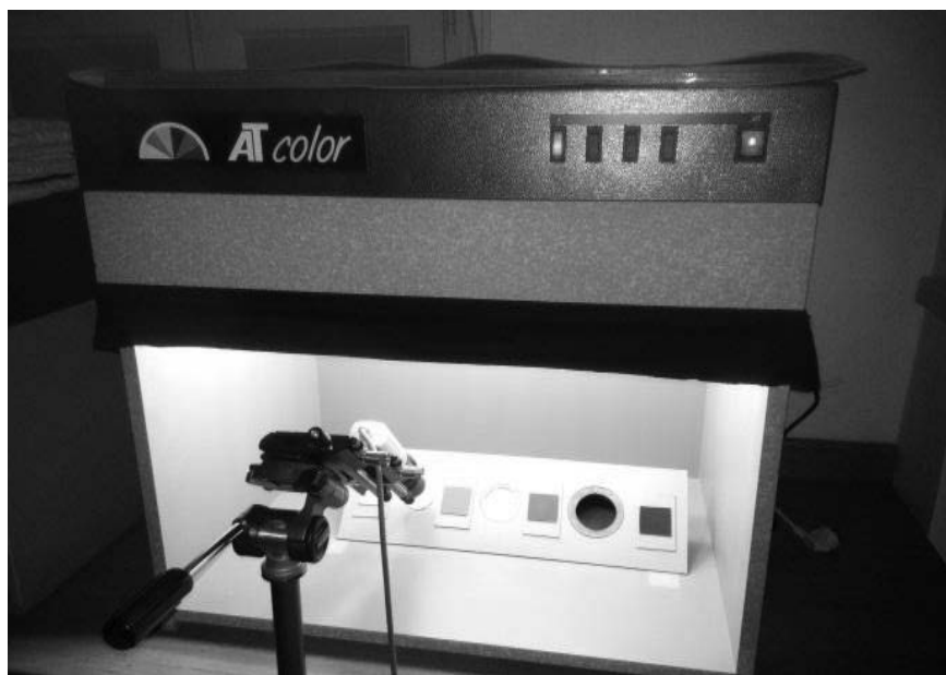
Figure 1. AT color light cabinet (equipped with Violet Chip White LEDs) and Konica Minolta CA-210 used for colour measurement with non-contact method.
