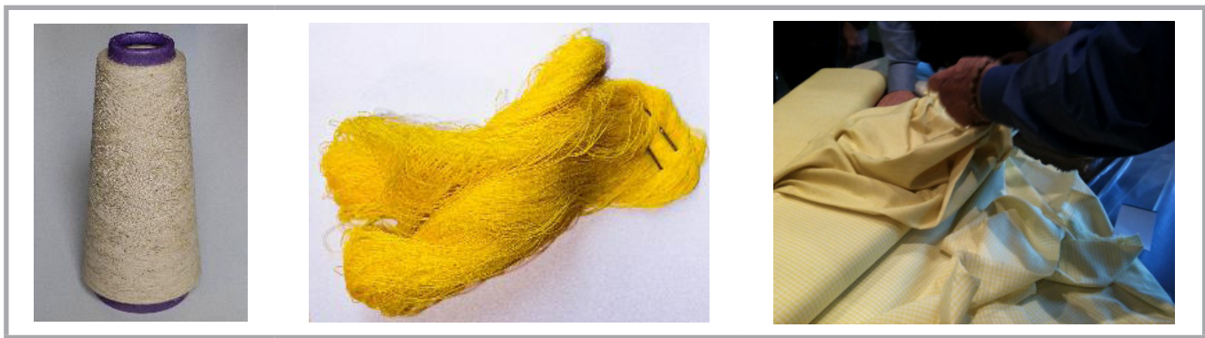
Figure 1. Yarns and textiles made of Spartium junceum fibres.
