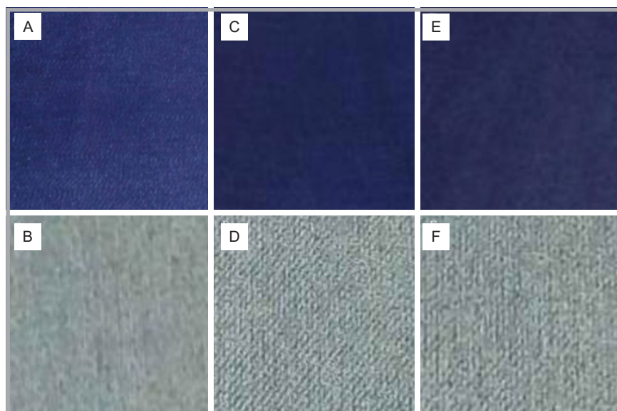
Figure 3. Photographs of denim samples; A: sample 1, B: treated sample 1, C: sample 2, D: treated sample 2, E: sample 3, F: treated sample 3. P = 240 \text{ W} , V = 10000 \text{ mm/min} .
