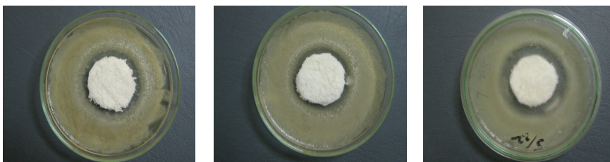
Figure 5. Zone of inhibition after 10 washing cycles of samples A-10, N-10 and HCAN-10.
