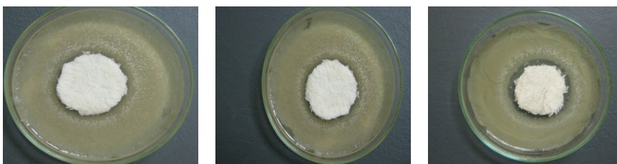
Figure 6. Zone of inhibition after 20 wash cycles of samples A-10, N-10 and HCAN-10.
